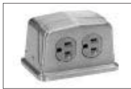
The 1993 NEC bans face-up outlets from countertops. Tombstone outlets, such as this one from Walker, are an acceptable alternative.
