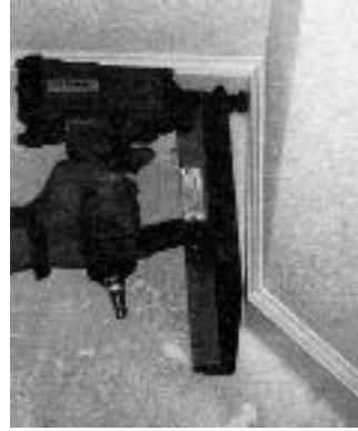
A nailer with an angled magazine (left) is easier to use at inside corners. A parallel magazine (right) can get in the way in tight spaces.
