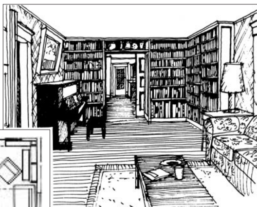
Figure 3. In the TV/guest room, a custom pocket door (made from two doors doweled together at their edges) slides behind the built-in bookcases to provide privacy.
