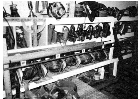
Power tools are shelved on the left side of the truck, near the rear for easy access. Custom-cut shelves brace the tools against motion.
