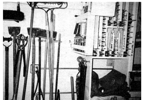
Long-handed tools are toward the front of the truck on the right side. Caulks and glue tubes are easily accessible from a custom-made rack.
