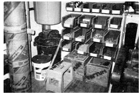
Nails and screws rest in open bins at the truck's front, clearly labeled, so nail bags can be quickly loaded or unloaded.
