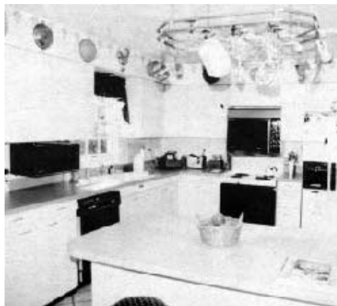
To reduce the use of formaldehyde-containing fiberboard, the kitchen uses high-gloss metal cabinets instead of veneered fiberboard. The counters are plastic laminate, glued with low-toxic adhesives to solid wood substrates.
