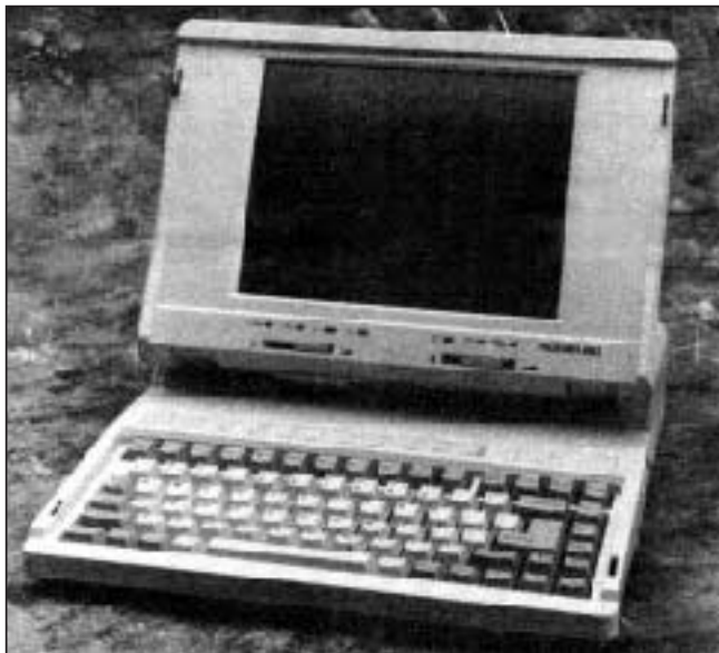
Figure 1. The Packard Bell PB286LPV, at about 15 pounds, is relatively heavy for a laptop but its weighty batteries provide more time on line without recharging than most models.
