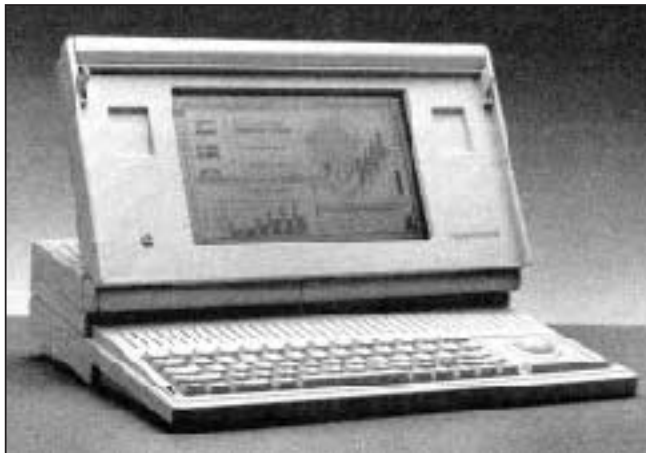
Figure 2. Apple's "luggable" Macintosh Portable offers excellent power and memory; and ports for a printer, mouse, modem, and extra drives, monitor, and speaker.
