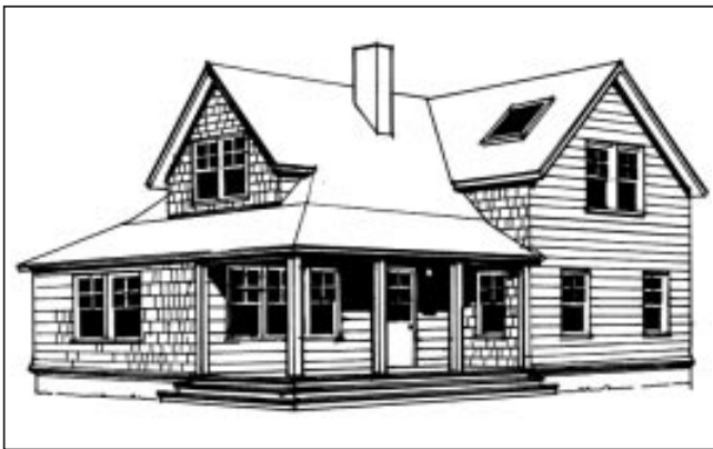
Figure 4. In this shingle-style house, the cross gables erupt from a basic "background" hip roof.
