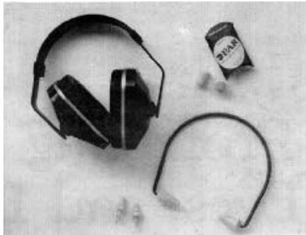
Take your pick of hearing protection (clockwise from top left): Earmuffs provide good, convenient protection, but are bulky. Moldable foam earplugs provide excellent protection, but are inconvenient for intermittent use. Canal caps, which fit over the head or under the chin are lightweight and convenient and offer modest protection. Pre-molded plugs (also available attached to cords) can work well if you get a good fit.
