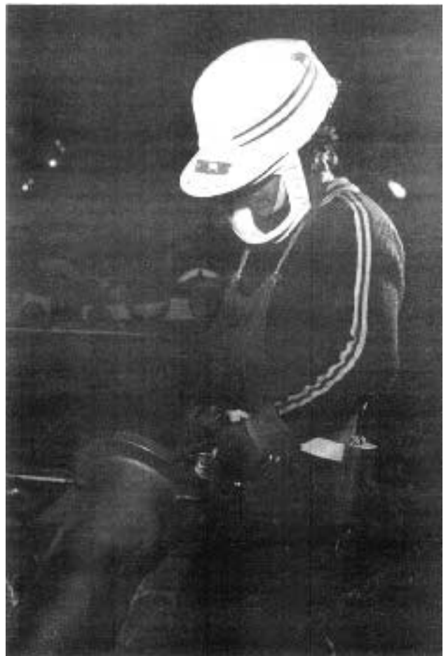
Bearded workers have few options for dust protection. One possibility is 3M's Airhat system (W-316), which uses a built-in fan to blow filtered air into the helmet. Because of the pressurized air, a tight fit to the face is less critical, but the beard must still fit inside the face seal says 3M.
