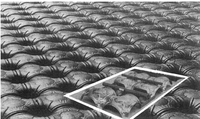
The "Airfloor" system by Aircontrol Systems makes use of metal forms (shown here) over which a concrete slab is poured. The forms provide channels for forced hot air to heat the slab.
